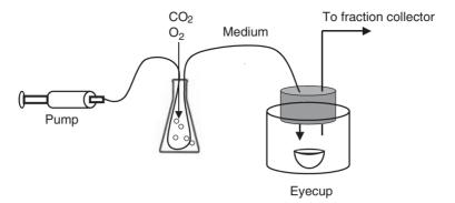
**Figure 4.6.** Diagram of the Xenopus eyecup preparation. Culture medium is supplemented with 5-hydroxy-L-tryptophan in order to detect melatonin from a single eyecup. The medium is gassed with CO<sub>2</sub> and O<sub>2</sub>, and then delivered to a superfusion chamber containing the eyecup. The perfusate is delivered to a fraction collector for quantifying concentrations of melatonin. [Adapted from Anderson and Green (2000): *Microsc Res Tech* **50**: 360–372.]
